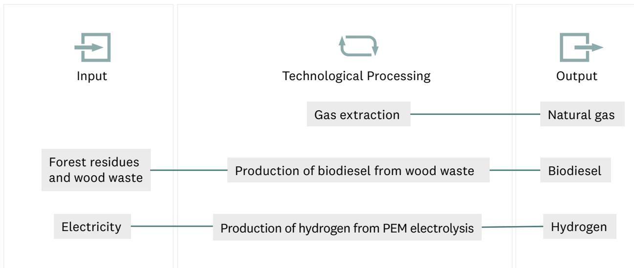
Figure 22: Examples of technological processes described in TIMES-NZ. “Gas extraction” is a primary energy supply process and thus it does not require an input fuel in TIMES. The other two examples describe the conversion of an input commodity (fuel) into a more useful output.
